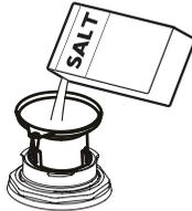
Place the supplied funnel over the mouth of the salt container, then put 1.5 kg of salt in the container.
